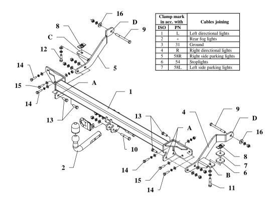
This towbar is designed to assembly in following cars: FIAT DUCATO (L1, L2, L3), PEUGEOT BOXER (L1, L2, L3), CITROEN JUMPER (L1, L2, L3), metal built-up, produced since 2006, catalogue no. R39 and is prepared to tow trailers max total weight 2500 kg and max vertical load 120 kg.
